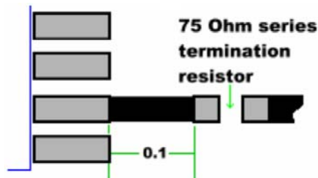
Figure 4. 75\Omega Series Resistor 0.1 Inches from Pin
